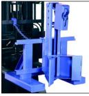
**Model 288-1** is designed to handle 1 drum.
