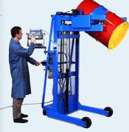
Model 515-T-114 Has 60" pour height, is scale-equipped with intrinsically safe indicator, and has air power lift and tilt.
