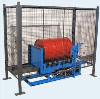
Hydra-Lift Drum Roller shown with Controls, and Guard Enclosure with Safety Interlock to meet OSHA requirements
