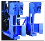
**Model 288-2-2H** handle 1 or 2 drums at a time with two heads per drum.
